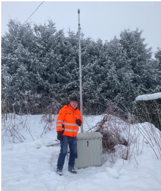
Oslo Airport's NTMS records the aircraft noise level continuously at 11 sites around the airport.
