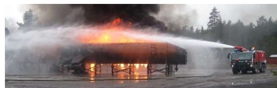
Use of fire-fighting foam has led to the large concentrations of PFOS in ground and groundwater at Oslo Airport.
