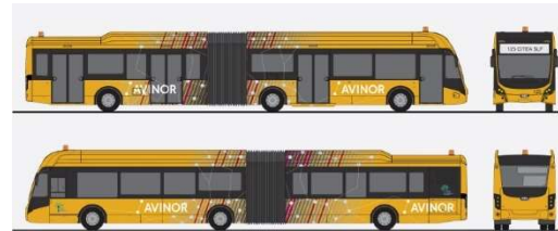
Oslo Airport's airside buses will look as shown in the picture above. Due to visibility requirements on the aircraft side, the buses are yellow.
